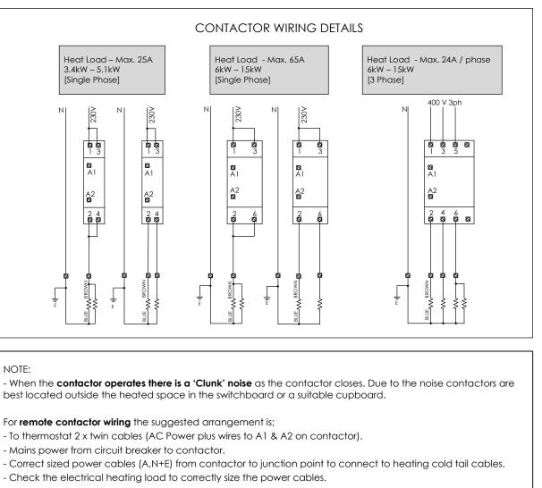
NOTE: Earth screen of all heating cables is to be connected to EARTH
