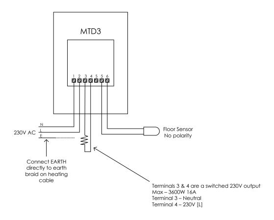
NOTE: Earth screen of all heating cables is to be connected to EARTH
