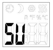
This option provides a read-out containing the software number.
