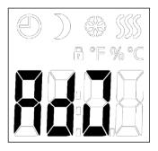
This option allows you to calibrate the measured room temperature.
