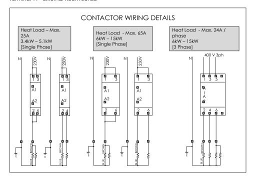
NOTE: Earth screen of all heating cables is to be connected to EARTH
